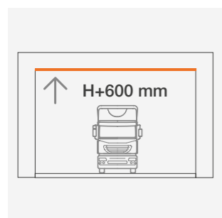
Ⓐ Architrave dimension H + 600 mm
